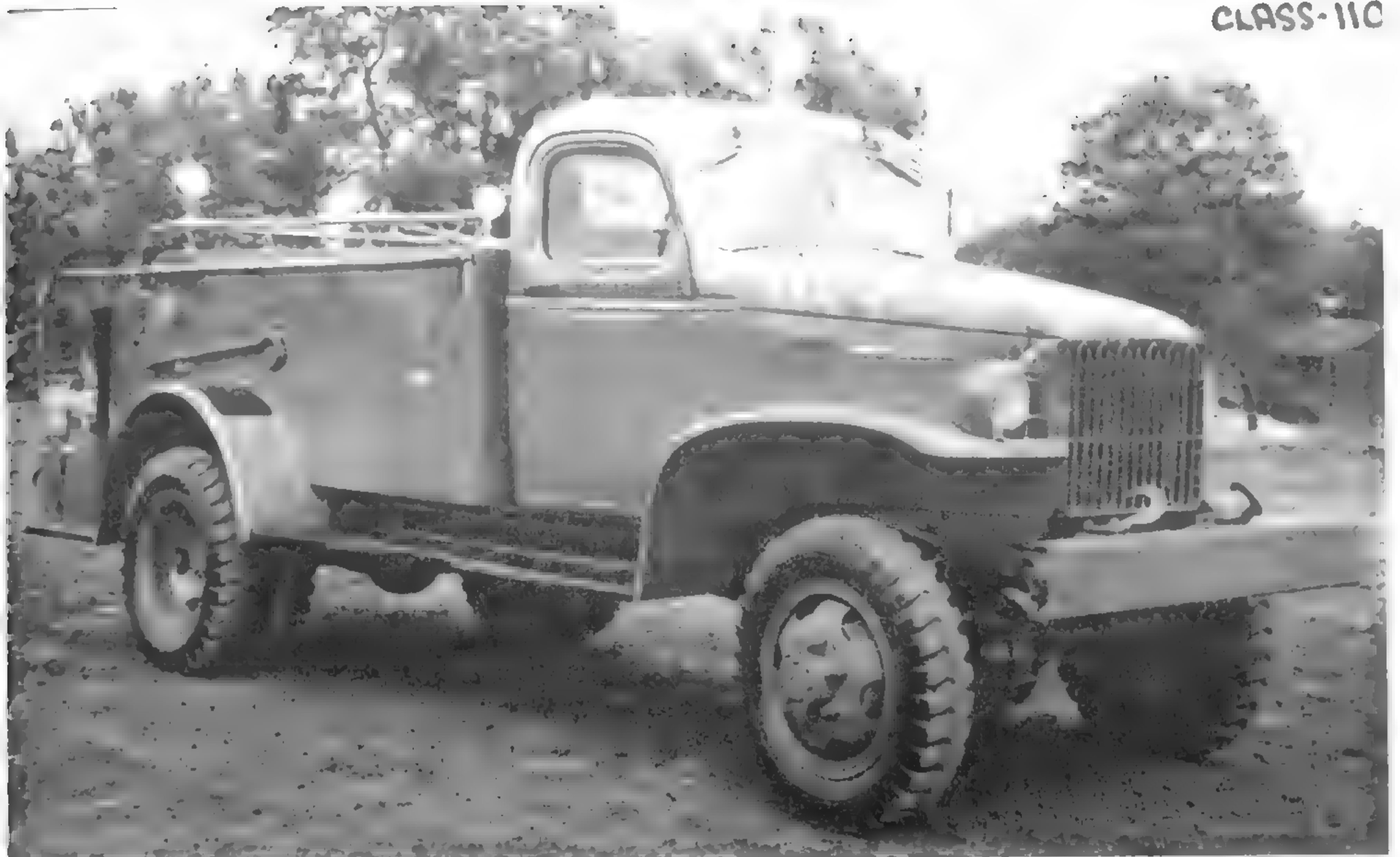
This is one of many types of fire trucks built on the G-506 chassis. The nameplate on the side of the hood says Model 110-QMC. This truck was designed to discharge foam, and the hose reel was mounted at the rear behind the large foam tank that constitutes the bulk of the bed. Even though the truck itself is marked as a 110 in this period photo, this very same truck, U.S.A. registration number W-50702, is shown in the April 1949 ORD 3 SNL G-1 supply catalog, and is identified in that publication as a Class 135. (Photo from the Richard Adelman Collection)
